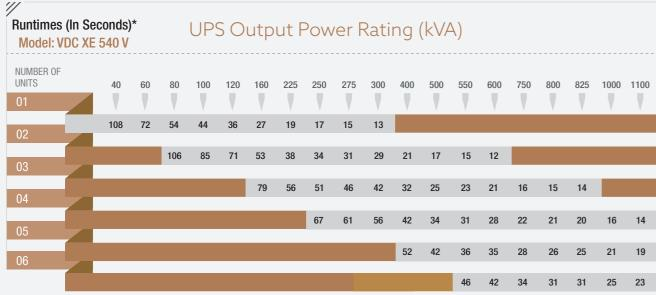
\*Backup times are typical using .9 Output Power Factor, 100% Full Load Rating, 96% UPS Inverter Efficiency and minimum 540 voltage bus setting.
